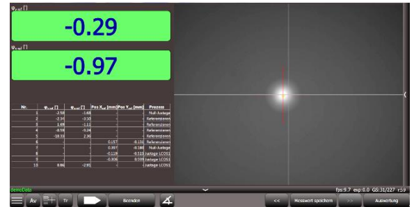
Fig.: Angular measurement with plane mirror
