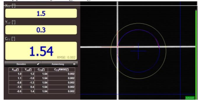
Centering measurement with tolerance field circle
