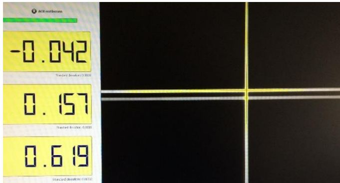
Fig. 1: Wedge angle measurement in reflection via double cross; measured wedge angle is 0.619 wmin = 37.14 wsec.
